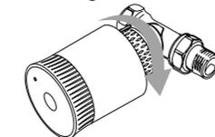
If the valve connection in your home does not match the controller, install the accessories first
